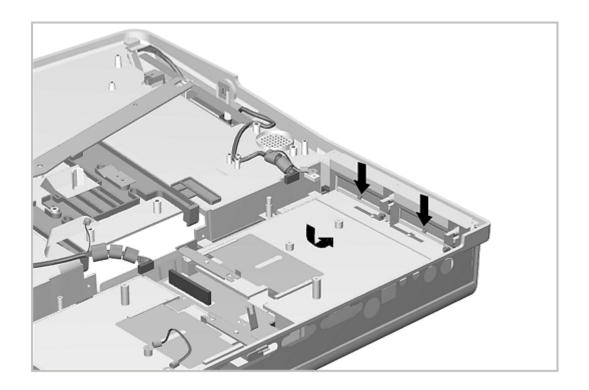
Figure 7-24. Installing the MultiBay Assembly
